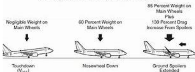
Effects of Nosewheel Contact and Ground Spoilers On Weight-on-wheels and Aerodynamic Drag
