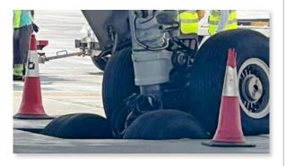
An engineer on site said that the drain cover collapsed as the main gear taxied over it, resulting in it falling in, dismissing rumors that the cover was missing. <u>Click here to read more.</u>
